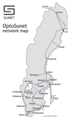
Figure 3.4: The OptoSUNET network consists of leased fibre, and is divided into three separate systems: north, west and south. Each of the systems have two separate networks called "red" and "green" such that each site has at least two access paths. Image: SUNET, Börje Josefsson.
